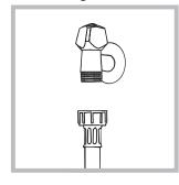
1. Connect the supply pipe by screwing it to a cold water tap using a 3/4 gas threaded connection (see figure). Before performing the
